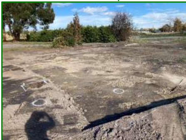
Photos 10-11: Eastern area of heavy metal contamination with XRF test locations
